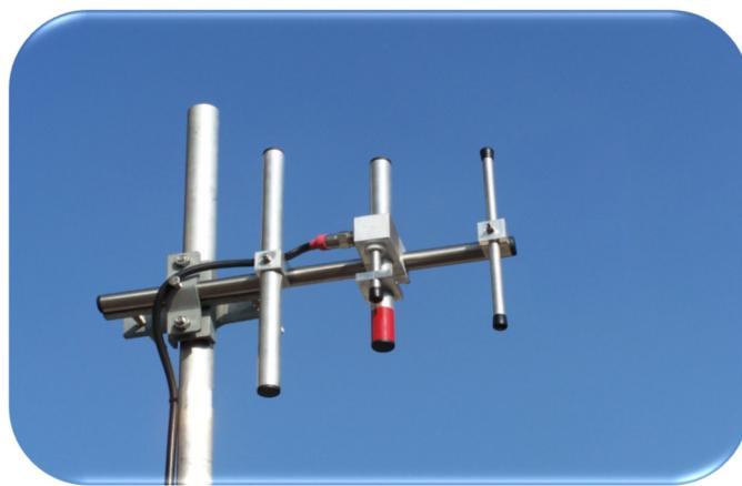
■ UHF NARROW BAND YAGI ANTENNA
